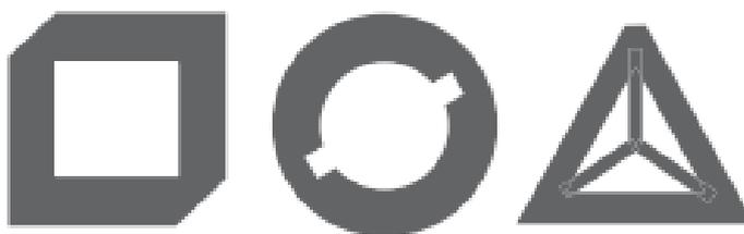
Gambar 2.6 Model Geometri *Patch* Antena Polarisasi Sirkular [19]
