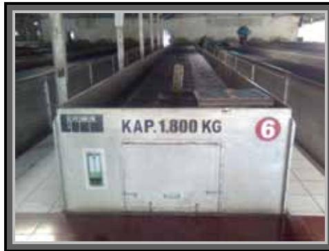
Gambar 4.19 Withering Trough
