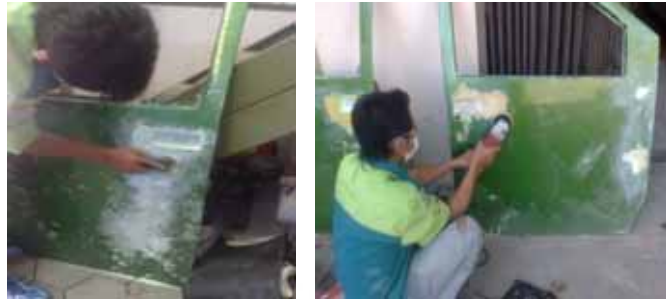
Gambar 3.21. Proses pengamplasan
