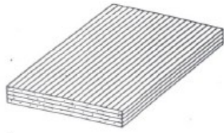
(a) Continuous fiber composite
