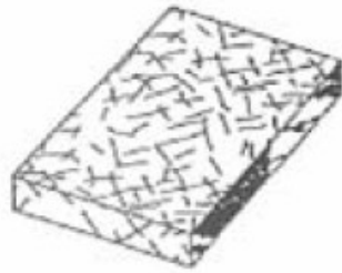
(c) Discontinuous fiber composite (chopped fiber composite)
