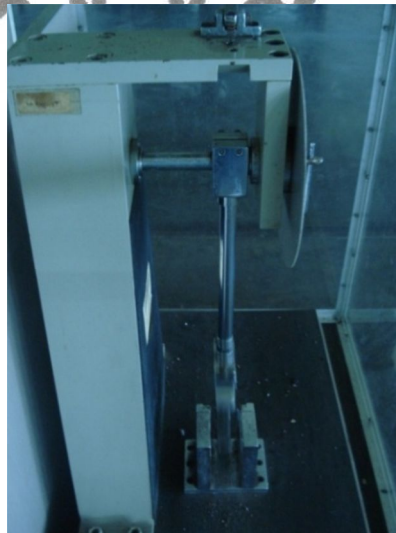
Gambar 3.2. Alat Uji Impak Charpy Sanata Dharma Sumber : Pengamatan, 2011
