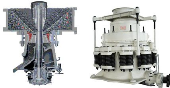
Gambar 2.9. Cone crusher ( http://www.mine-engineer.com dan www.iconcrusher.org )
