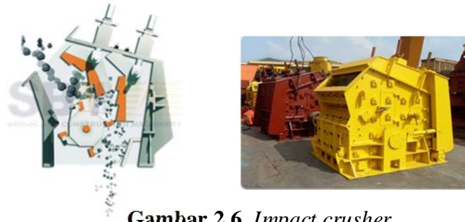
Gambar 2.6. Impact crusher ( www.iconcrusher.org dan www.sbmcrusher.com )
