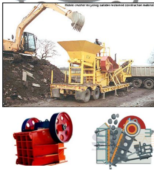
Gambar 2.5. Jaw crusher ( www.mine-engineer.com dan www.indonetwork.co.id )
