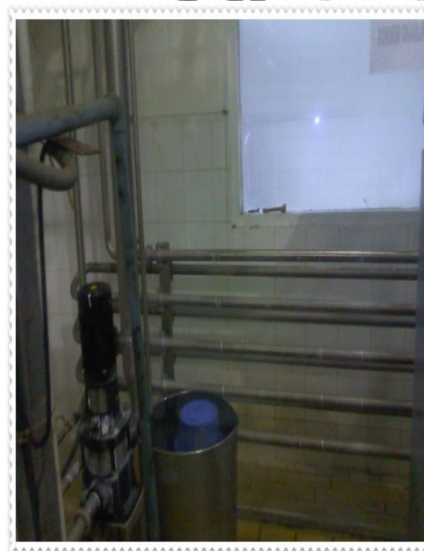
Gambar 4.15a Holding Tube
