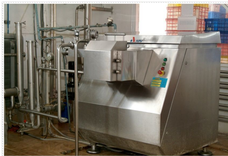
Gambar 4.13 Homogenizer
