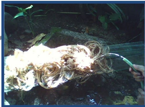
Gambar 3.9. Pencucian serat rami
