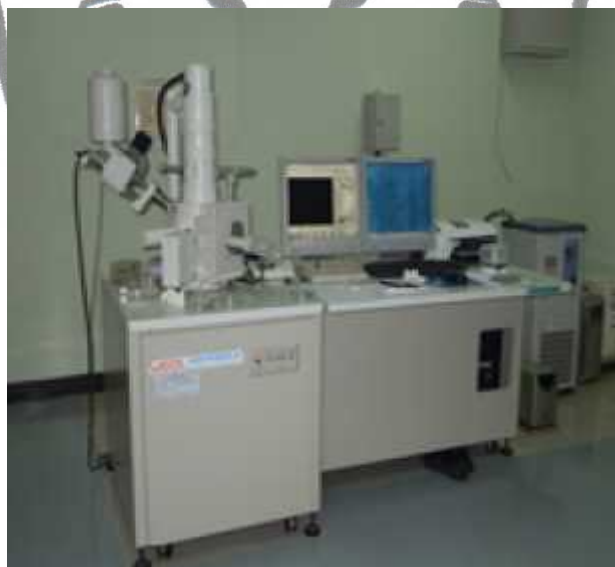
Gambar 3.15. Karakterisasi Scanning Electron Microscopy (SEM) merk JEOL seri JSM6360LA
