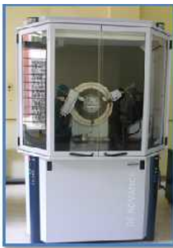
Gambar 3.14. Karakterisasi X-Ray Diffraction (XRD) merk Bruker model D8 ADVANCE
