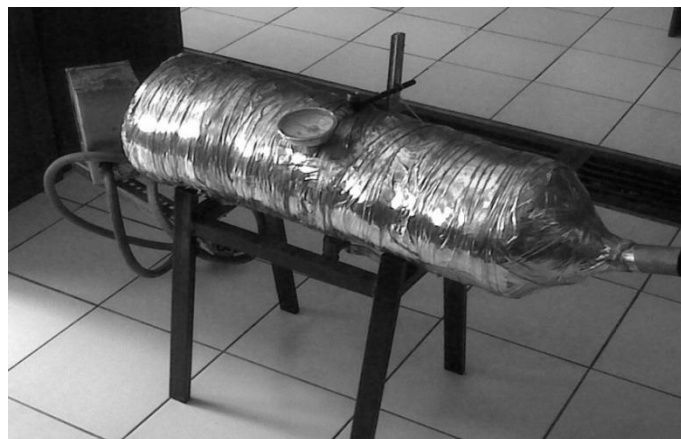
Gambar 4.2. Rangkaian Evaporator Tampak Samping
