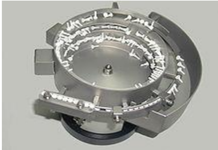
Gambar 2.12 Vibration Feeder
