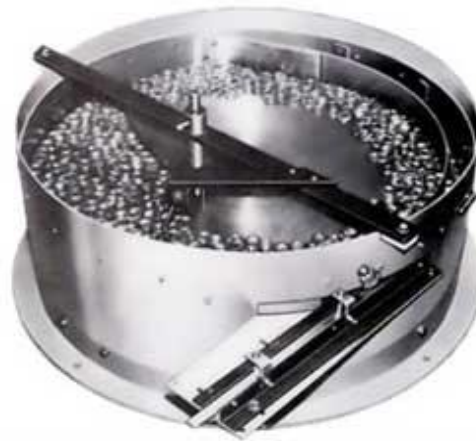
Gambar 2.13 Rotary Feeder
