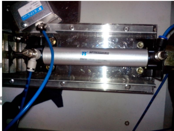
Gambar 2.2 Silinder Pneumatik Double Acting
