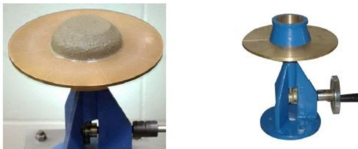
Gambar 2.1. Alat Uji Slump Flow
