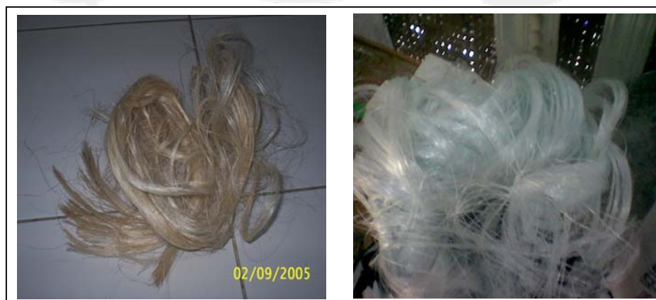
(a) (b) Gambar 2.4 (a) Serat agave cantula roxb, (b) serat rowing
