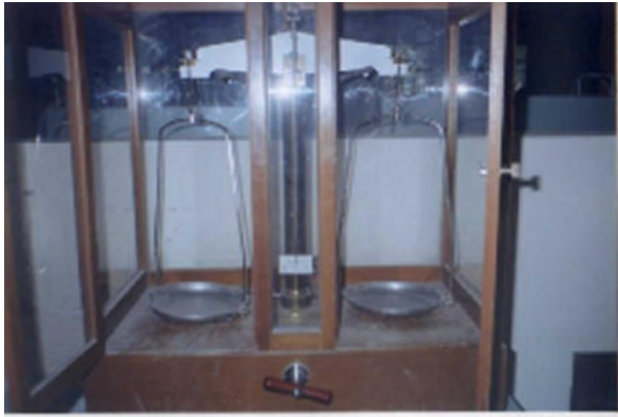
Gambar E.3 Neraca Merek Murayama Seisakusho Ltd Japan Kapasitas 5 Kg
