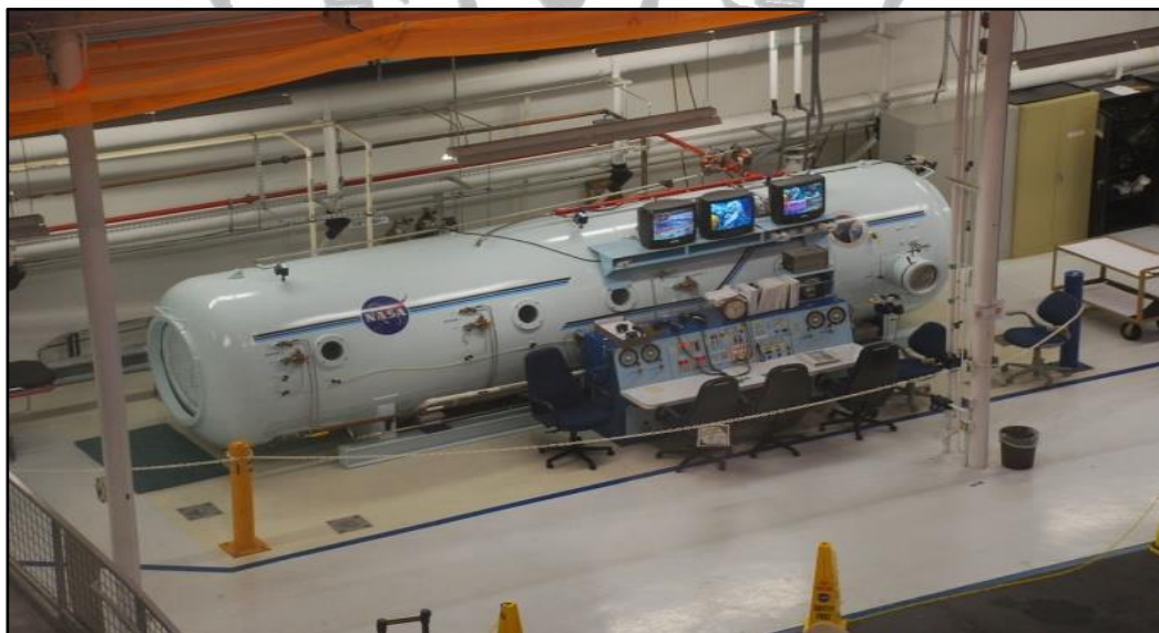
Gambar 3. Large Multipartmen Chamber
