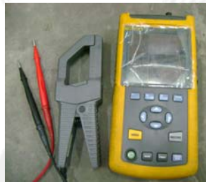
Gambar 3.7. Fluke Power Quality Analyzer
